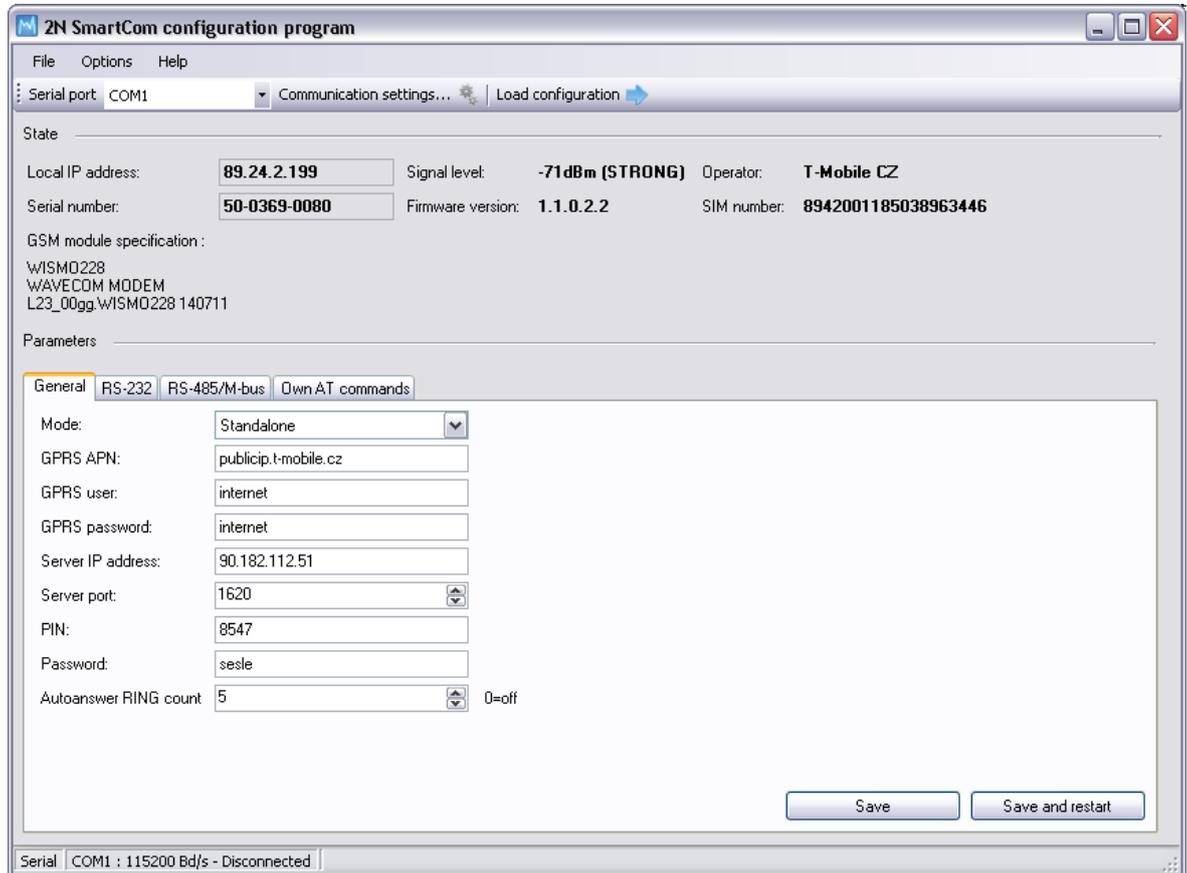
This is the 2N® SmartCOM Terminal Configuration Program (hereinafter referred to as Terminal Config only) window. Select the **Serial port** in the main toolbar for connection to 2N® SmartCOM (hereinafter referred to as the terminal). This list includes all available serial ports installed in the PC on which the application is running.
