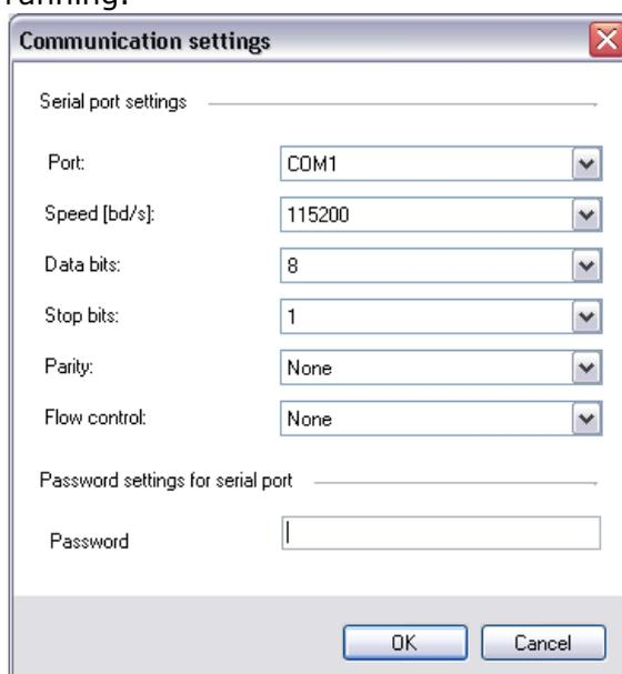
Having selected a port, use the **Communication settings** to adjust the communication speed and define signal transmission for the serial port. The 2N® SmartCOM factory values are set here by default. Refer to Fig. 5.2.
