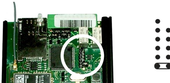
Disconnect 2N<sup>®</sup> SmartCOM from the power supply. Connect the jumper as shown in Fig. 5.1 and reconnect the power supply. Now the Flash memory is deleted and the factory default values are reset for all ports. Remember to remove the jumper to avoid deletion of the factory values upon every start.
