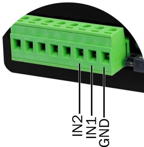
The input circuits can work in three modes - voltage, current or logical levels - as configured.
